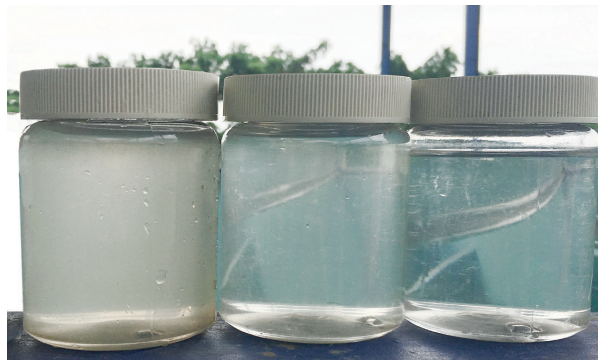
The first influent of Purification plant (River water) Raw water of Fiber Discfilter (Supernatant from Lamella) Treated water (Fiber Discfilter)
