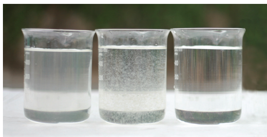
Raw water (River water) Flocculated water Treated water (Fiber Discfilter)
